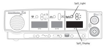
NOTE: If you are not monitoring oxygen saturation levels, the LCD display shows "OFF."
