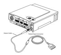
Step 3: Connect the Lead Wires to the ECG Patient Cable.
