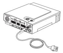
CAUTION: Do not twist or turn the oximeter patient cable to remove it from the SmartMonitor 2 PS as this may damage the
